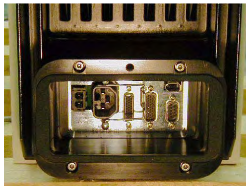
Figure 10-3. Cable Seal Housing Installed
