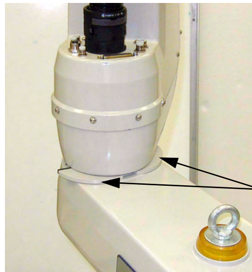
Figure 6-21. Joint 2 Adjustable Hardstop Locations
