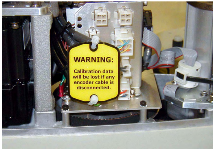
Figure 2-3. Warning Label on Encoder Cables
