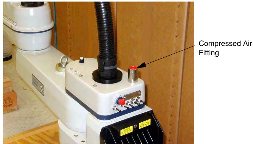
Figure 10-11. Compressed Air Fitting on Robot
