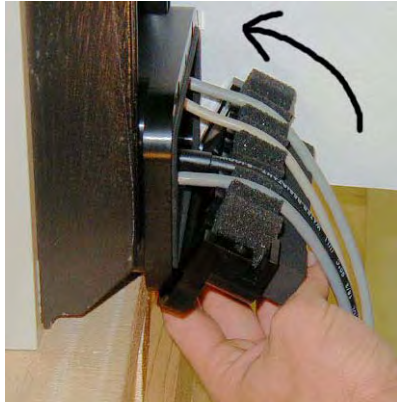
Figure 10-4. Installing Lower Flange
